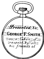
Fig. 177—Laying out letter by starting from the line.
