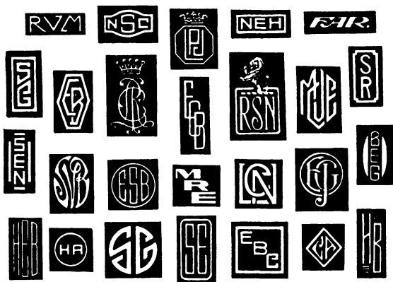
Fig. 218—Some styles of piercing used by G. M. Betser and Co. Ltd. Ties between letters, and letters and frame are not shown.
