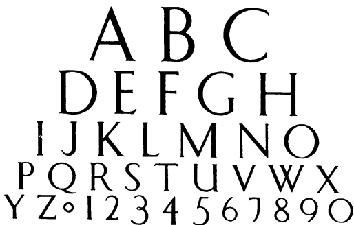
Fig. 188—A definite scale for each line gives an even graduation.
