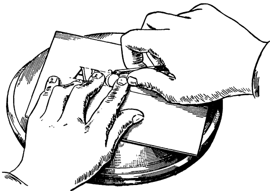
Fig. 36—Correct positions of the hands and fingers for engraving. Note that the index finger of the left hand presses against the thumb which is the turning fulcrum.
