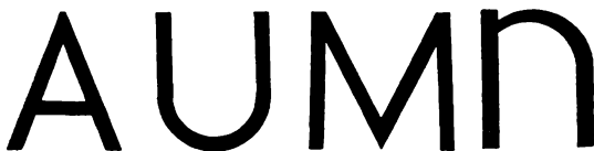
Fig. 198—Sans serif letters. The lower-case n at the end has been thinned where the curve butts into the upright.
